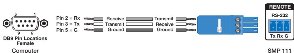
Figure 4. RS-232 Wiring Diagram
