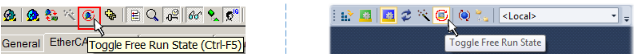
Fig. 169: TwinCAT can also be switched to this state by using a button (left: TwinCAT 2; right: TwinCAT 3)
