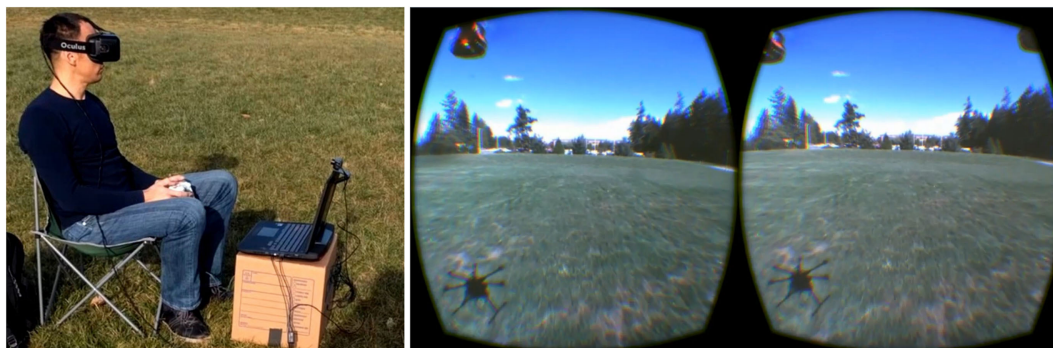
FIGURE 3 | (Left) Ground station setup. Operator flying a drone via our first person view system: GT control, oculus head-mounted display. (Right) The flight view from the operator perspective. Watch Movie S1 in Supplementary Material to see the setup at work.
