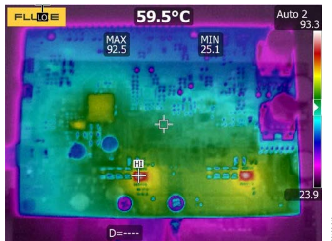
Figure 11. Thermal Image of EVAL-CN0508-RPIZ at 30 V Input, 2.75 A Current-Limit Output into 4 \Omega Load
