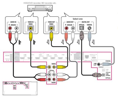
In order to record, you must connect the analog audio cables (the digital connection is for playback only) (page 71).
