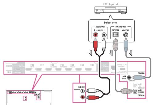
If your turntable has line-level outputs (i.e., it has a built-in phono pre-amp), connect it to the ANALOG IN 1 (CD) inputs instead.
