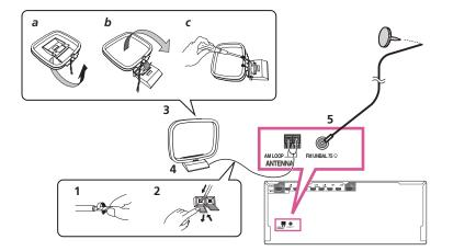
1 Pull off the protective shields of both AM antenna wires.
