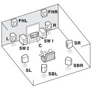
A 7.2 ch surround system connects the left and right front speakers (L/R), the center speaker (C), the left and right front height speakers (FHL/FHR), the left and right surround speakers (SL/SR), the left and right surround back speakers (SBL/SBR), and the subwoofers (SW 1/SW 2).
