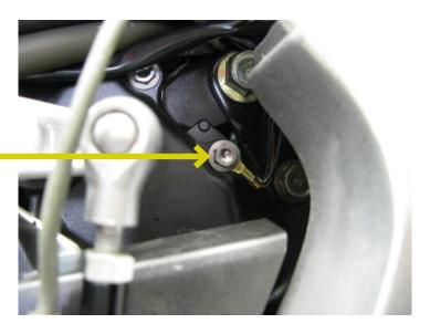
5. Continue to route the fuel harness along with the factory harness, forward to the TPS sensor which is located on the left side of the throttle bodies. Unplug the fac-
