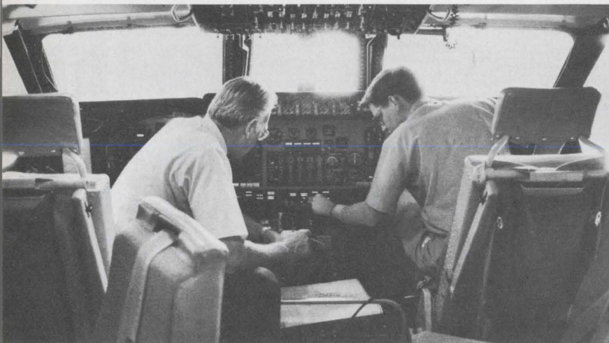
Flight crew compartment seats six—two pilots, navigator, engineer, and two observers. Upcoming tests will concentrate on the instrument landing system, radar altimeter, inertial navigator and engine readings. The display for the plane's automatic test system is at the lower right of the engineer's console (above).
