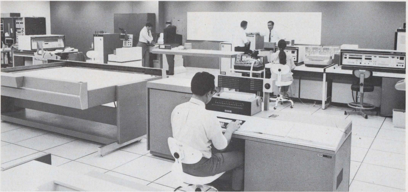
Fairchild's computer-aided design system will do the layout and generate test programs for the customer's
