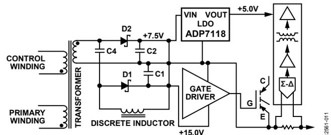
Figure 11. Dual Output Supply Supporting 15 V for the Isolated Gated Drive and 5 V for the Isolated Modulator
