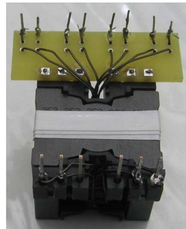
Figure 17. Prototype Flyback Transformer with Bobbin Extender
