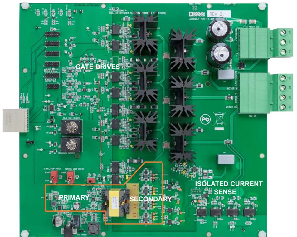
Figure 19. 3-Phase Motor Control Inverter with Bias Supplies
