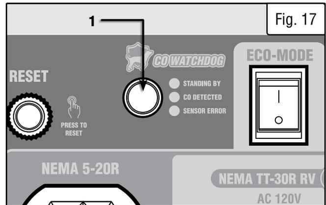
**NOTE:** if the generator is oriented so that the engine exhaust is blown towards the CO sensor, the generator may shut down.
