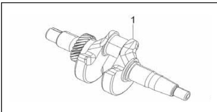
**Fig. 4 - Crankshaft Assembly**
