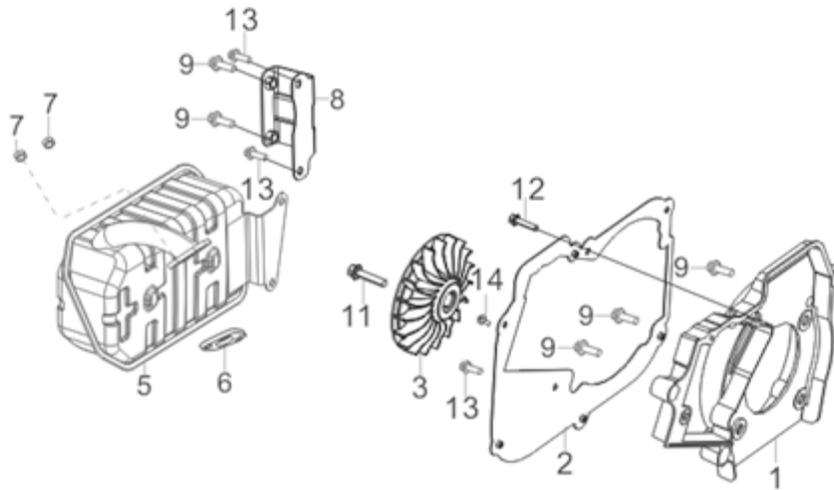
**Fig. 11 - Muffler Assembly**
