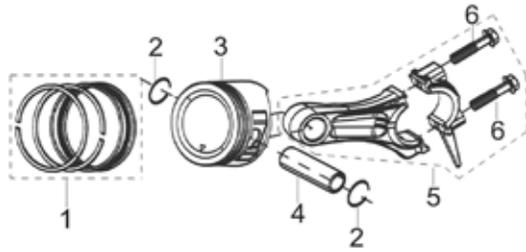
**Fig. 5 - Piston Ring Set & Connecting Rod**
