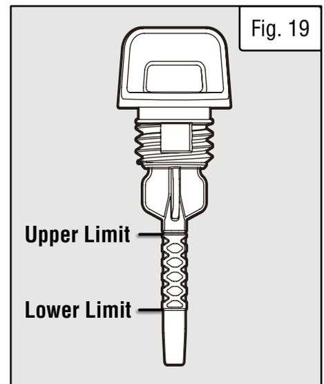
**TIP:** Your WEN generator is compatible with the WEN 55201 Magnetic Oil Dipstick (not included), available for purchase at [wenproducts.com](http://wenproducts.com). The dipstick's industrial-strength magnetic tip will collect metal shavings from your generator's oil pan to help preserve the engine and extend your generator's lifespan.
