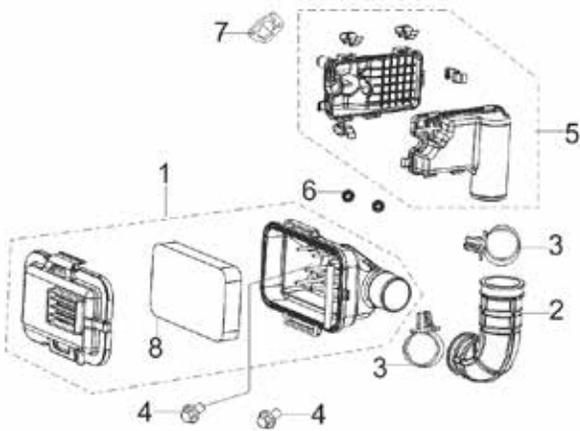
**Fig. 10 - Air Filter Assembly**
