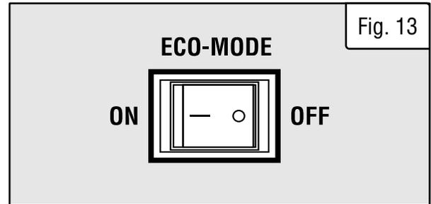
Keep this switch engaged **ONLY** when the power load requirement is less than 2550W (75% of the rated watts). Do not engage the Eco-Mode Switch when the total load is more than 2550W. The generator engine must run at full speed to supply power for anything over 2550W.
