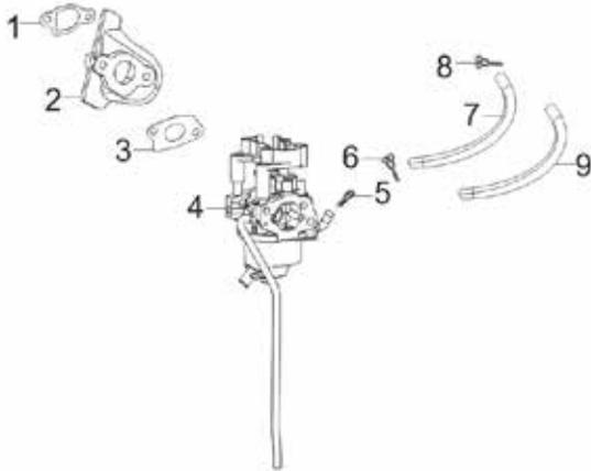
**Fig. 8 - Carburetor Assembly**
