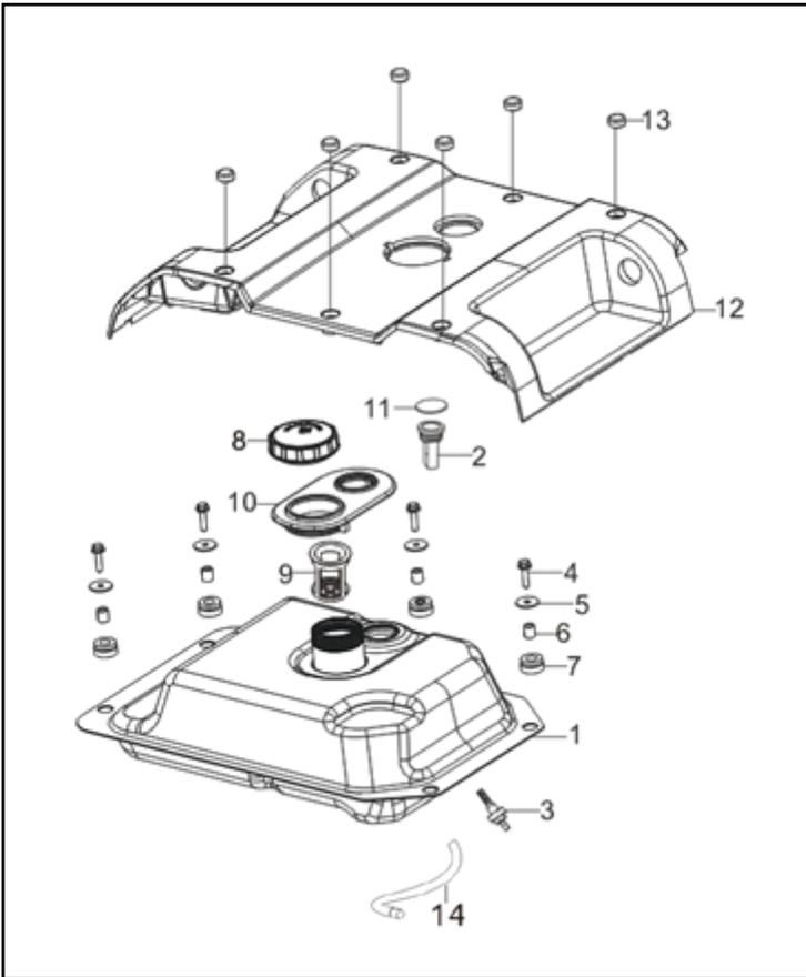
**Fig. 12 - Fuel Tank Assembly**
