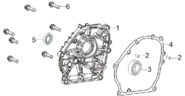
**Fig. 2 - Crankcase Cover Assembly**
