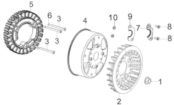
**Fig. 9 - Rotor/Stator Assembly**
