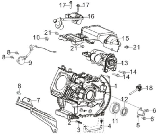
**Fig. 1 - Crankcase Assembly**
