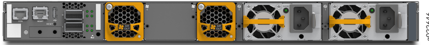
Figure 12: Rear View of an EX4400-48T and EX4400-48P Switch with AC Power Supplies
