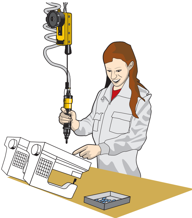
Bench assembly of small electric devices is a typical application for screwdrivers supported in balancers.
