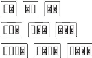
1. Carefully cut out the template below along the dashed line that represents the appropriate multiple gang application. Cut along the solid line to provide clearance for any existing controls. Temporarily attach the template to the wall at the desired mounting location.
