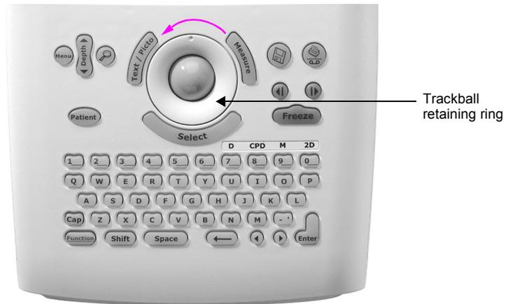
**Figure 7.9** Removing the Trackball Retaining Ring
