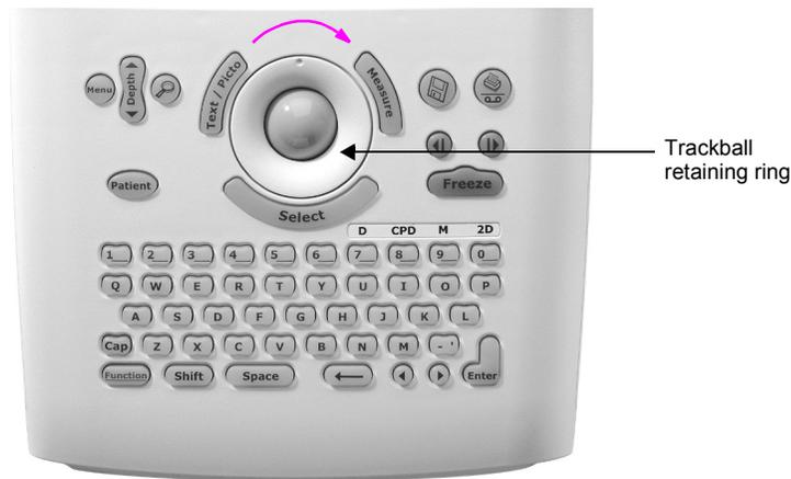
**Figure 7.15** Installing the Trackball Retaining Ring
