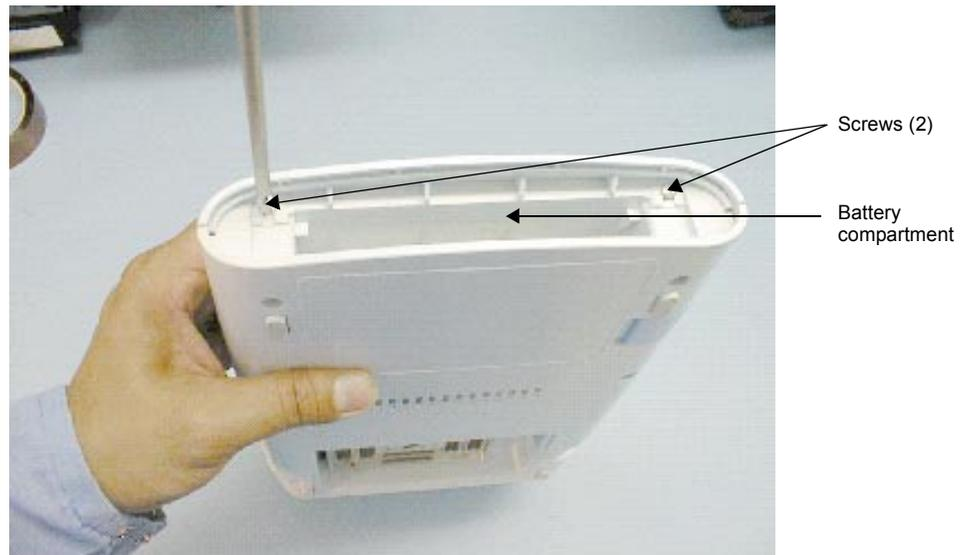
**Figure 7.8** Replacing the Control Panel Subassembly
