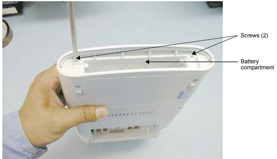
**Figure 7.6** Removing the Control Panel Subassembly
