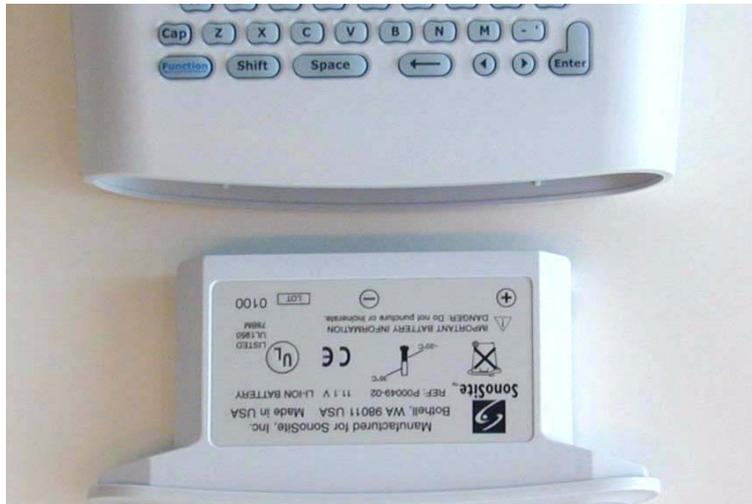
**Figure 4.2** Inserting the Battery
