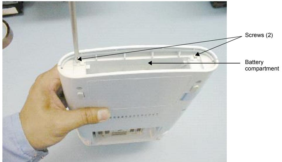
**Figure 7.17** Replacing the Control Panel
