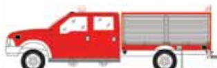
DARLEY VISION WILDLAND WL004 (CAFS Option Included) Pump (HE500 BS 39K) 450 Gallon Tank Copolymer StakPak Body
