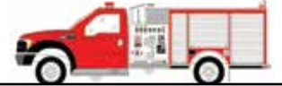
DARLEY VISION INITIAL ATTACK IA011 (CAFS Option Included) Pump (1000) 350 Gallon Tank Copolymer Attack Body
