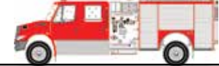
DARLEY VISION INITIAL ATTACK IA010 (CAFS Option Included) Pump (1000) 500 Gallon Tank Copolymer Attack Body
