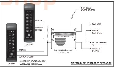
The User Manual of the DA-2800 provides the operation details of the system on decoding controller mode and independent operation mode. Please contact your local agent if purchase of the DA-2800 Controller is required. **REMARK:** DA-2801 is the simplified version of the DA-2800 without wireless remote control function.
