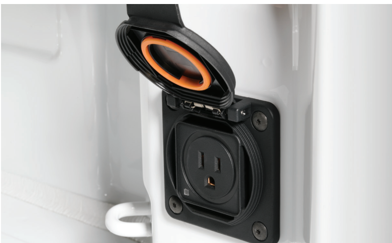
Standard 120-volt power outlet in bed
