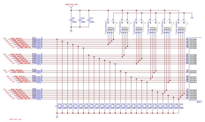
Figure 4. Partial Schematic Showing Default R and C values
