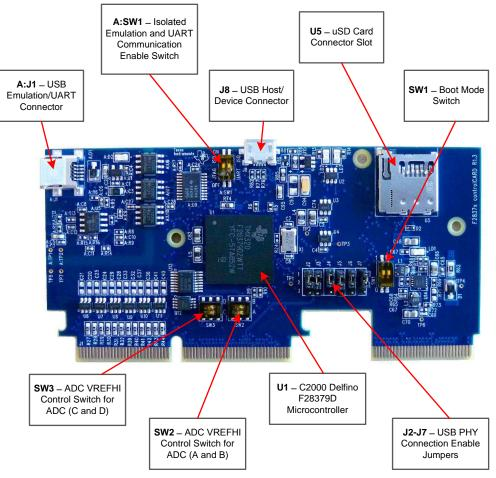
Figure 6. Key components on the controlCARD
