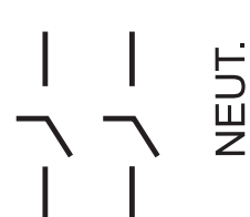
Three-wire SN, 120/240 Volts AC, No Fuse
