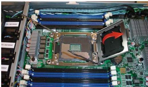
4. Remove the protection cap from the CPU socket.
