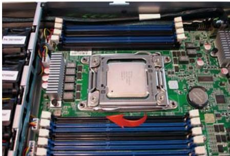
8. Position the heatsink on top of the CPU and secure it with 4 screws.
