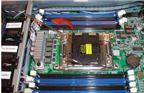
3. Lift the CPU socket cover to a fully open position.
