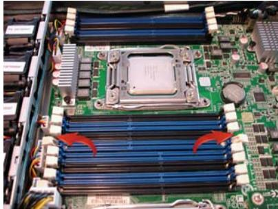
3. Align and insert the memory module down onto the slot. When inserted properly, the memory slot locking levers lock automatically on the indentations at the ends of the module. Follow the recommended memory population table to install the other memory modules.
