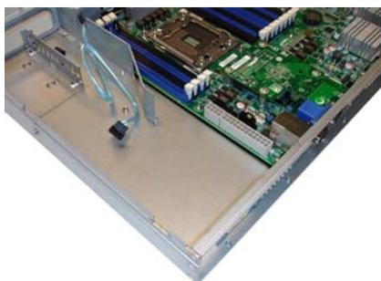
4. After replacing a new power supply, follow Step 1~3 in reverse order to reinstall the power supply.
