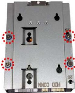
7. Place the HDD tray into the chassis.
