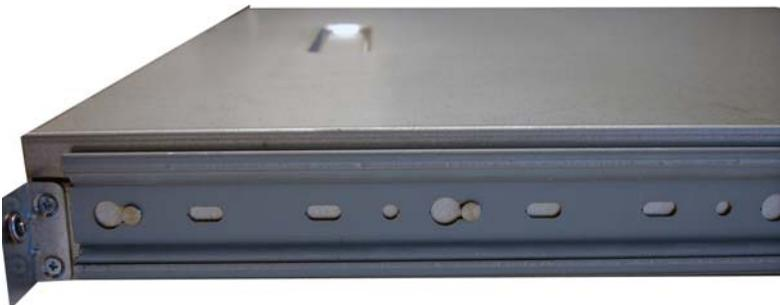
4. Align the inner sliding rail on the other side of the server.
