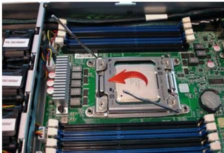
7. Press the levers down to secure the CPU.
