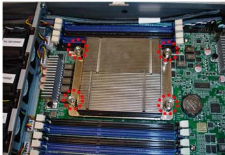
9. Repeat steps 2 to 8 to install the second CPU and heatsink.
