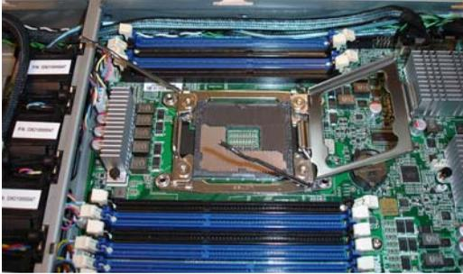
5. Place the CPU into the socket making sure that the gold arrow is located in the right direction.
