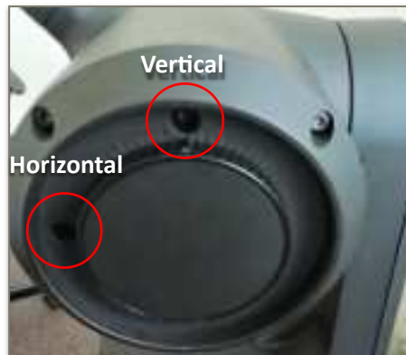
2. Use the hex key to turn the screw (in this example the vertical screw)
