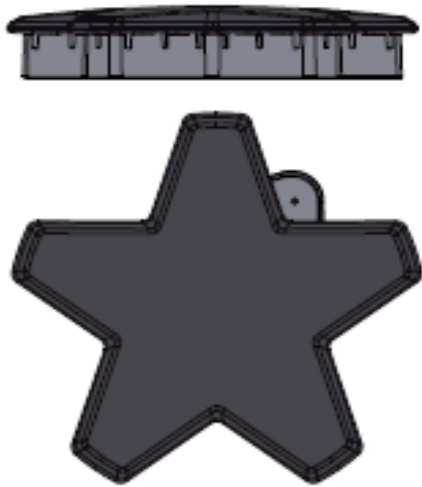
Figure 14: Correct Burner Cap Placement
