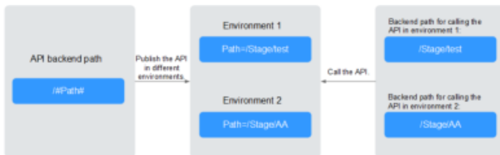
Figure 5-3 Application of environment variables
