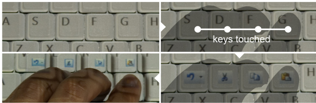
Figure 9. A group of four commands (e.g., undo, cut, copy and paste) can be assigned to the user's finger tips. Whenever the fingers touch a row of adjacent keys, the underlying keys are overloaded accordingly.
