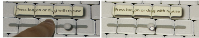
Figure 6. Continuous controls (such as sliders) can be operated in discrete steps using the keys, or at finer resolution using the mouse.
