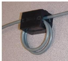
Figure 34 - Fair-Rite Filter Installed on RS-485 Communication Line
