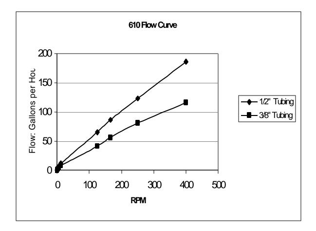
Flow curve established with water and a minimum lifting distance. Flow will be affected by fluid viscocity and lift distance.
