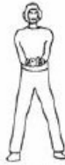
SPEED BRAKE EXTEND ARMS AT WAIST WITH PALMS TOGETHER. KEEP WRISTS TOGETHER AND OPEN PALMS.
