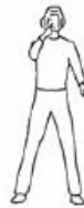
ENGAGE NOSE GEAR STEERING POINT TO NOSE WITH INDEX FINGER WHILE INDICATING DIRECTION OF TURN WITH OTHER INDEX FINGER.
