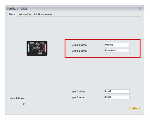
It is not normally possible to assign names to the inputs, only to the outputs in order to identify in the programming which output controls which lighting.
