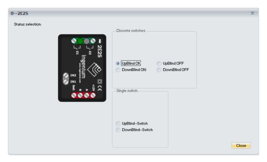
Closing first relay is chosen (output 1 ON).
