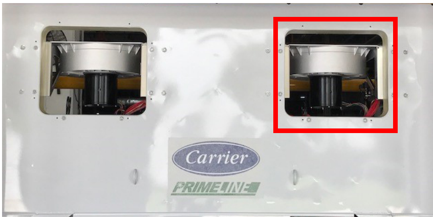
Figure 7.19 Removing Evaporator Motor
