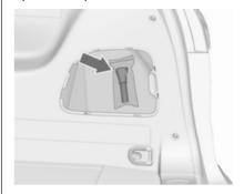
The funnel is located on the righthand side storage compartment in the load compartment.
