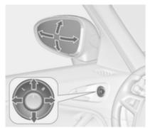
Select the relevant exterior mirror by turning the control to left **(L)** or right **(R)**. Adjust respective mirror by tilting the four-way control.
