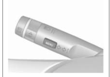
Press **MENU** to switch between the menus or to return from a submenu to the next higher menu level.
