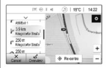
To display a turning manoeuvre on the map, scroll through the list and touch the desired manoeuvre. The map jumps to the respective location on the map.
