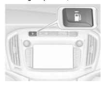
Pressing witches between petrol and natural gas operation. Switching is not possible at high loads (e.g. powerful acceleration, driving at full throttle). The LED status shows the current operating mode.
