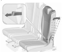
Pull the loop, adjust inclination, release strap and allow backrest to engage.
