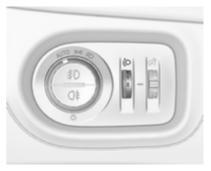
To adapt headlight range to the vehicle load to prevent dazzling: turn thumb wheel ∮ to required position.
