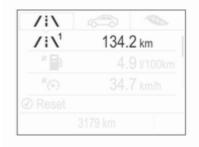
Trip odometer counts up to 9999 km and then restarts at 0.
