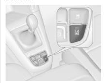
The lane departure warning system is activated by pressing 14. The illuminated LED in the button indicates that the system is switched on. When the control indicator 14 in the instrument cluster illuminates green, the system is ready to operate.
