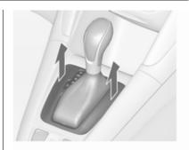
Release the selector lever trim from the centre console at the front, fold it upwards and rotate it to the left.
