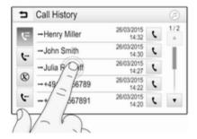
Touch a screen button or menu item. The corresponding system function is activated, a message is shown, or a submenu with further options is displayed.
