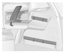
Install the hooks in the desired position in the rails: insert the hook in the upper groove on the rail and press in the lower groove.
