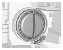
Rotate cap anticlockwise and remove it.
