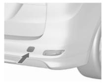
Wrap a cloth around the tip of a flat screwdriver to prevent paint damage. Insert a screwdriver in the slot at the lower edge of the cap. Release the cap by carefully moving the screwdriver downwards. To prevent damage it is recommended to place a cloth between the screwdriver and the frame.
