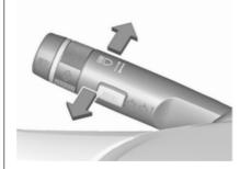
Push lever to switch from low to high beam.
