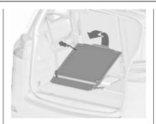
Pull up the seat by the upper loop, fold out and allow seat to engage in upright position.
