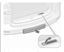
Pull release lever up. The rear carrier system disengages and travels quickly out of the rear bumper.
