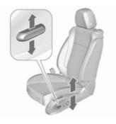
Move switch upwards/downwards.
