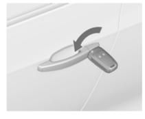
Manually unlock the driver's door by turning the key in the lock. Switch on the ignition and press to unlock all doors, load compartment and fuel filler flap. By switching on the ignition, the anti-theft locking system is deactivated.
