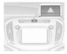
Operated by pressing <u>A</u>. In the event of an accident with airbag deployment the hazard warning flashers are activated automatically.
