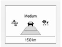
Note that the alert timing sensitivity setting is shared with the following distance setting of the adaptive cruise control. So changing the alert timing sensitivity changes the adaptive cruise control following distance setting.
