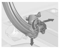
Open the protective flap and turn the key to position a to unlock the coupling ball bar.
