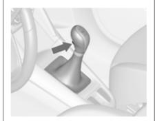
To engage reverse, depress the clutch pedal and then press the release button on the selector lever and engage the gear.
