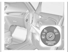
The front passenger airbag system can be deactivated via a keyoperated switch on the passenger side of the instrument panel.
