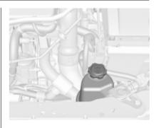
Power steering fluid level normally does not have to be checked. If an unusual noise sounds during steering or the power steering reacts unusually, seek the assistance of a workshop.
