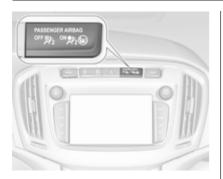
If the control indicator ON ₹2 illuminates for approx. 60 seconds after the ignition is switched on, the front passenger airbag system will inflate in the event of a collision.
