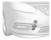
Disengage cap at bottom and remove downwards.
