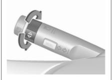
Turn the adjuster wheel to select a submenu of the main menu or to set a numeric value.
