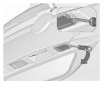
Insert screwdriver in recess of the cover, press to the side and release spring. Remove cover.
