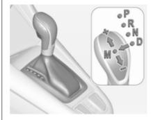
P: park position, wheels are locked, engage only when the vehicle is stationary and the parking brake is applied
