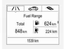
Display of the approximate total fuel range and for each fuel tank (LPG or CNG and petrol). A low fuel level in either tank is indicated by **Low** in the respective section.
