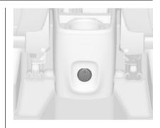
Further 12 Volt power outlets are located in the rear console
