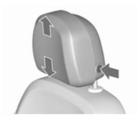
**Height adjustment**Press release button, adjust height, engage.
