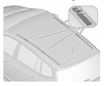
To fasten a roof rack, open the caps in the roof strips. Insert the mounting provisions, as instructed, in the retainer indicated in the illustration.
