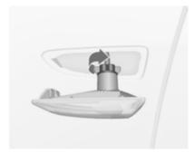
2. Turn bulb holder anticlockwise and remove from housing.
