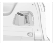
The funnel is located on the right side storage in the load compartment.
