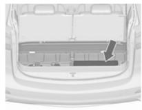
Stow the warning triangle in the storage of the load compartment floor in front of the tailgate.
