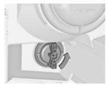
Rotate bulb socket anticlockwise to disengage. Withdraw the bulb socket from the reflector housing.
