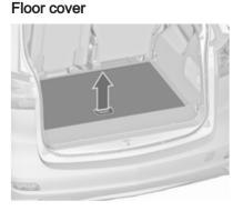
On versions without third seat row, there are storage boxes under the floor cover. To open lift up the cover and fold it upright behind rear seats.
