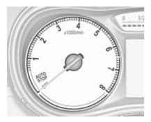
Displays the engine speed.
