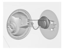
The fuel filler cap can be retained in the bracket on the fuel filler flap.
