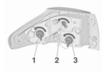
5. Remove and replace the bulb by turning the bulb socket.
