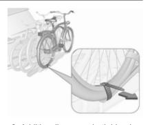
Additionally secure both bicycle wheels of the fourth bicycle to the wheel recesses using the tensioning straps.
