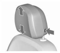
Press release button, adjust height, engage.
