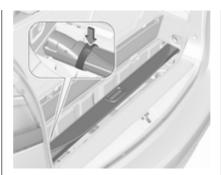
Fasten the load compartment cover in the storage with the Velcro tape.
