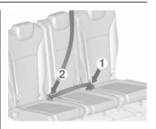
Remove lower latch plate from retainer and click it into left-hand buckle (1) at the centre seat. Guide the upper latch plate with the belt over the lap area and the shoulder (do not twist) and click into right-hand buckle (2) at centre seat.
