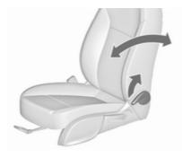
Pull lever, adjust inclination and release lever. Allow the seat to engage audibly.
