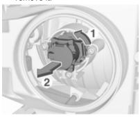
Rotate the bulb holder anticlockwise to disengage. Withdraw the bulb holder from the reflector housing.
