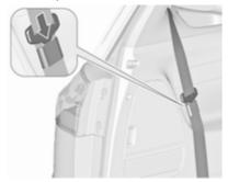
Insert the latch plate of the seat belt on each side into the pocket that is mounted at the belt.
