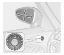
Select the relevant exterior mirror by turning the control to the left **(L)** or right **(R)**. Adjust respective mirror by tilting the four-way control.
