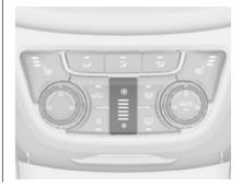
Press the lower button to decrease or upper button to increase fan speed. The fan speed is indicated by the number of segments in the display.
