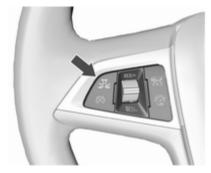
Press %; the current setting is shown in the Driver Information Centre. Press % again to change the alert sensitivity. The setting is also displayed in the top line of the Driver Information Centre.
