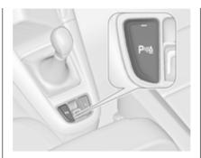
An illuminated LED in the parking assist button  $P^{n}$  indicates that the system is ready to operate.
