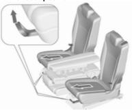
Pull the handle under each outer seat and slide seats to forward position.
