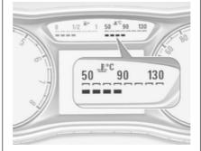
Number of LEDs displayed shows the coolant temperature.
