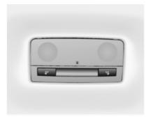
Illuminate in conjunction with the front courtesy light depending on rocker switch position.
