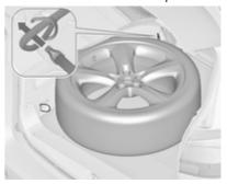
Place the loop end of the strap through the front lashing eye on the left side. 3. Place the hook end of the strap through the loop and pull it until the strap is fastened securely to the lashing eye.
