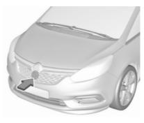
The radar unit is mounted behind the radiator grille below the brand emblem.
