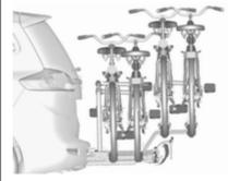
The rear carrier system (Flex-Fix system) allows two bicycles to be attached to an extendable carrier integrated into the vehicle floor. It is possible to attach two further bicycles on an adapter. The transportation of other objects is not permitted.
