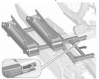
Attach the adapter to the rear carrier system as shown in the illustration.
