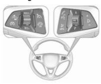
The Infotainment system, some driver assistance systems and a connected mobile phone can be operated via the controls on the steering wheel.
