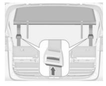
Push button on the tightener to release the strap on both sides. Detach hooks from the eyes. Unhook the safety net rods from the brackets in the roof frame. Roll up the net and secure with a strap.
