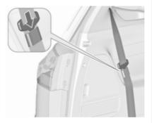
When seat belts are not used or when folding the seats, insert the latch plate of the seat belt on each side into the pocket that is mounted at the belt.
