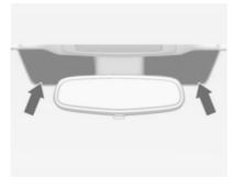
The marked areas on the windscreen are not covered with the coating. Devices for electronic data recording and fee payment must be attached in these areas. Otherwise data recording malfunctions may occur.
