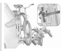
Guide the strap attached to the adapter underneath the lever to fold back the rear carrier system. Fasten the strap.
