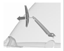
Lift wiper arm. Disengage wiper blade as shown in illustration and remove. Attach the wiper blade slightly angled to the wiper arm and push until it engages.
