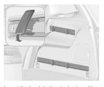
Insert the hook in the desired position first in the upper groove of the rail and then press in the lower groove. To remove, first pull out of the upper groove.
