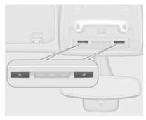
Operated by pressing \( \subseteq \) and \( \alpha \) in front and rear courtesy lights.
