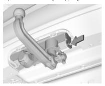
Attach breakaway stopping cable to eye.
