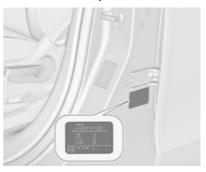
The identification plate is located on the front left or right door frame.
