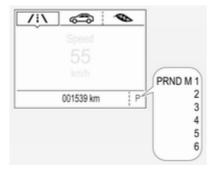
The mode or selected gear is shown in the Driver Information Centre. In automatic mode, the driving programme is indicated by **D**.
