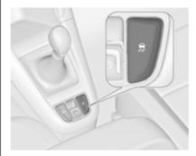
TC can be switched off when spinning of drive wheels is required: press \$ briefly.
