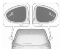
Side blind spot alert is active from speeds of 10 km/h up to 140 km/h. Driving faster than 140 km/h deactivates the system, indicated by low lighting warning symbols and in both exterior mirrors. Reducing the speed again will extinguish the warning symbols. If a vehicle is then detected in the blind zone, the warning symbols and will illuminate as normal on the relevant side.
