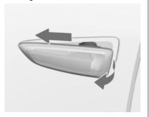
1. Slide lamp to its left side and remove with its right end.
