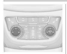
If the minimum temperature **Lo** is set, the climate control system runs at maximum cooling, if cooling **\*** is switched on.
