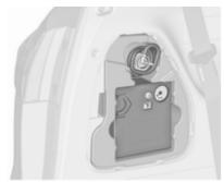
The tyre repair kit is on the left side in the load compartment behind a cover.
