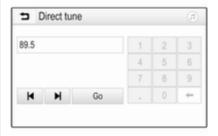
Enter the desired frequency. Use ← to delete digits entered. If necessary, touch ◄ or ► to subsequently adjust the input.
