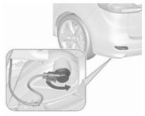
Turn the bulb socket anticlockwise and remove it from the reflector.
