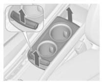
Pull the handle in front of cupholder and remove it vertically out of the console.
