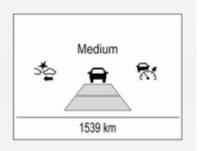
The selected following distance is indicated by filled distance bars on the adaptive cruise control page.
