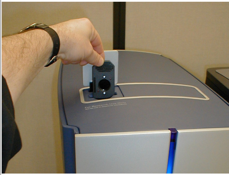
Figure 6.19 Removing the array
