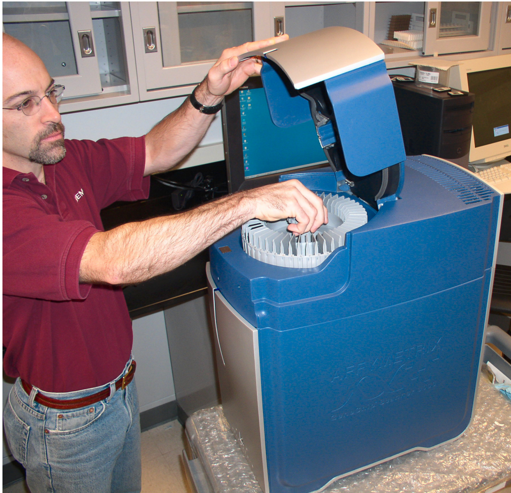
Figure 6.23 Inserting and turning the carousel; the carousel should be seated and flush with housing.
