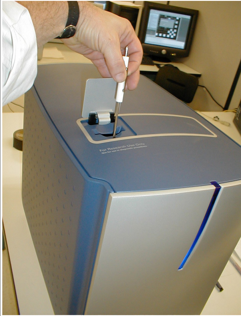
Figure 6.18 Turning the rescue screw
