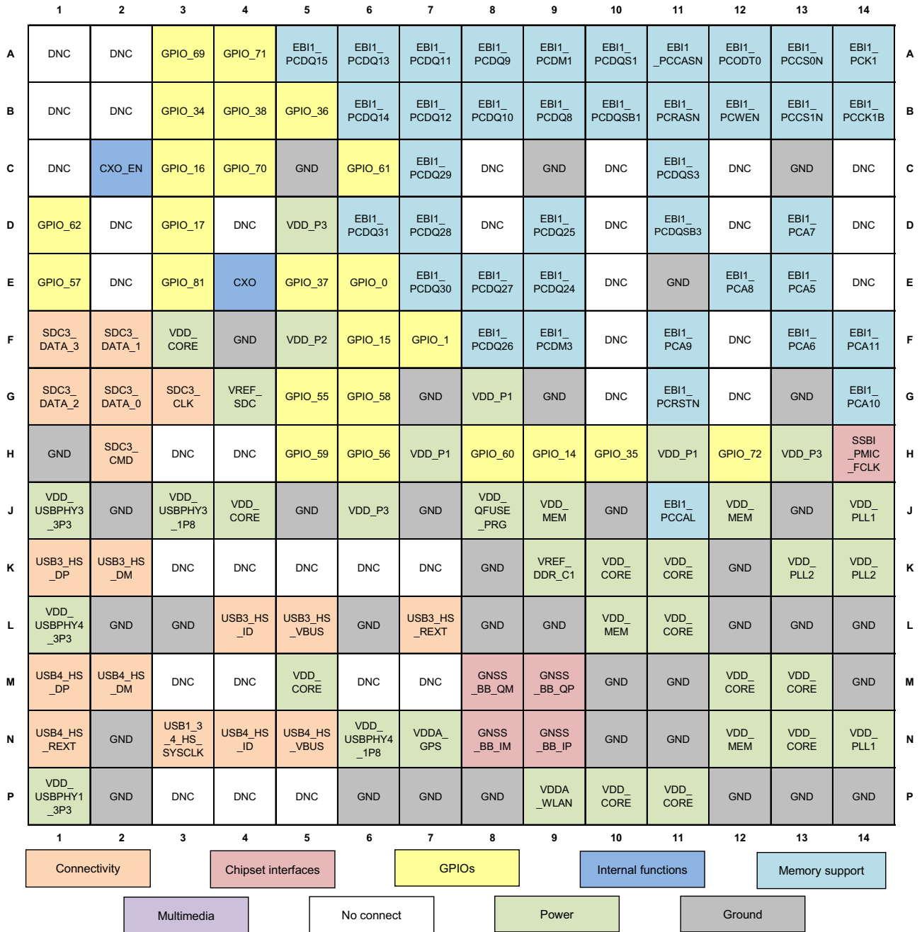
Figure 6-3 APQ8064 pin assignments – upper left quadrant
