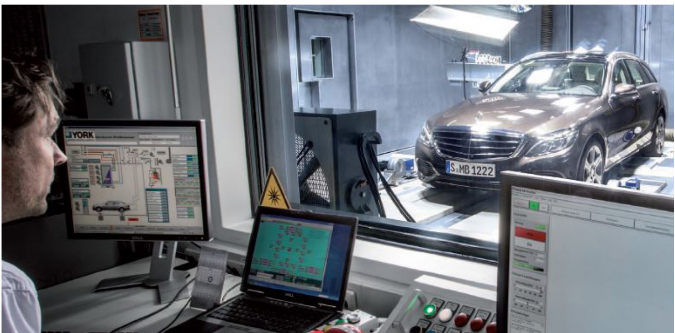
Figure 3-1: Test chamber to measure car cabin emissions
