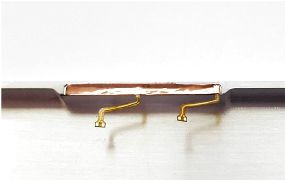
Figure 13. Copper Foil Shielded “Faraday Box”
