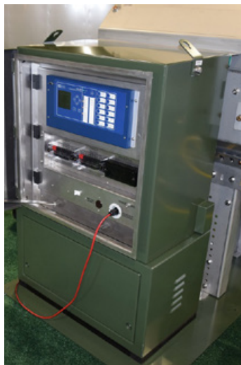
Figure 21. Schweitzer Engineering Laboratories SEL-451 integrated in exterior cabinet
