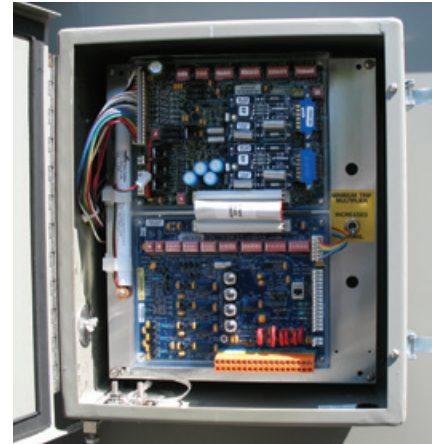
Figure 8. TPG control with SCADA shown.
