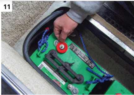
[10] While the cables are disconnected, clean the terminals with a wire brush as well. [11] In addition to preventing corrosion, felt terminal pads like this one are color coded, which makes it easier to discern the positive and negative terminals. [12] Once you've thoroughly cleaned the terminals and cables, apply a sparing amount of battery terminal protector spray or dielectric grease to prevent oxidation from forming on the bare metal.
