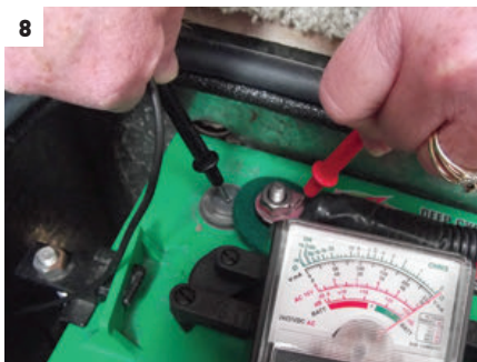
[7] Use the voltmeter function of the multimeter to verify that the battery or bank of two 6-volt batteries (shown) is charged; a fully charged battery will test at 12.7 volts. [8] Check the battery negative (-) post-to-cable connection by using the ohmmeter function of the meter, with one lead on the battery post and the other on the cable connector. [9] At the beginning of every season, detach the connection cables and clean with a wire brush.
