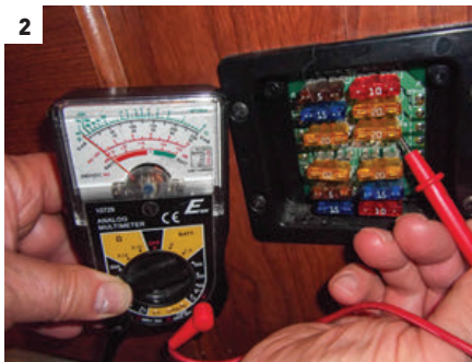
[1] A 10-watt bulb should read about 0.8 ohms resistance. [2] With the negative probe grounded, a fuse should read 12 volts DC on both sides. In this case, the fuse is blown so the meter reads 0 volts on the downstream side. [3] Along with a multimeter, a long wire with alligator clips on both ends is needed for testing ground connections.
