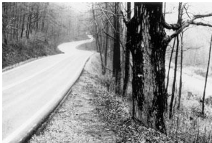
Figure A-6: Typical Roadway with Roadside Hazard Rating Equal to 6
