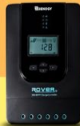
CHARGE CONTROLLER Regulates the energy from solar panels to charge service batteries.
