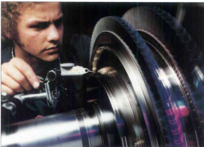
Testing the concentricity of the labyrinth seal webs on a turbine rotor.
