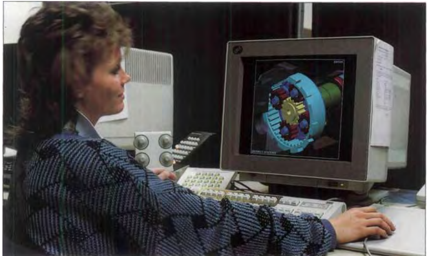
Kinematic simulation of planetary gear with the "CATIA/CAD/CAM" System.
