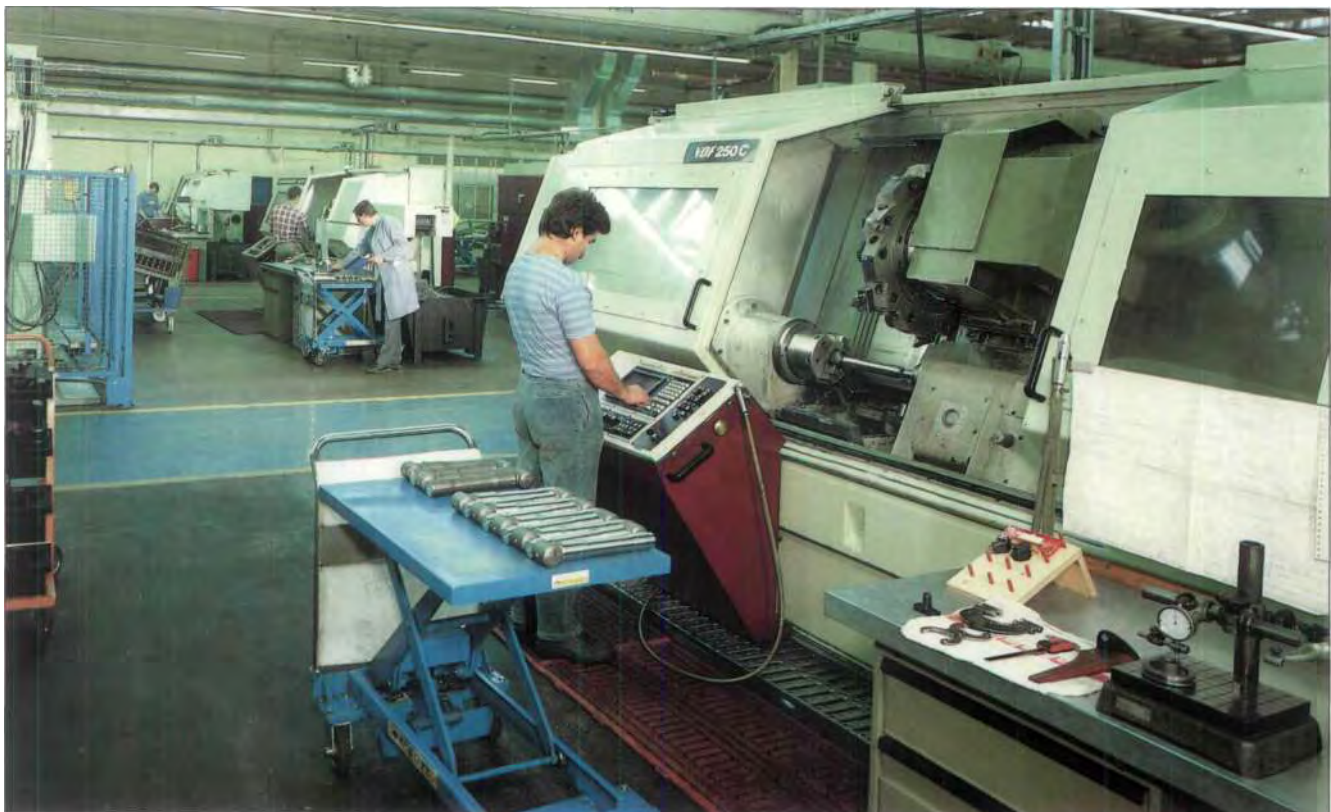
DNC lathe shop in the Berlin plant for manufacturing various production, pre-production and test pieces. Twenty-one CNC lathe machines, a tool setup device and a measuring machine are linked via a computer network system. Tasks formerly reserved for the planning department are now conducted by highly-skilled operators right on the production line,
