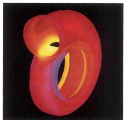
Ceramic turbine spiral housing: ceramic materials are used for the hot-gas conducting components employed in research on motor vehicle gas turbines. At temperatures of up to 1,300 degrees centigrade, high levels of thermal stress occur. This picture shows temperature distribution, ascertained with the help of computer simulation, in a turbine spiral housing.
