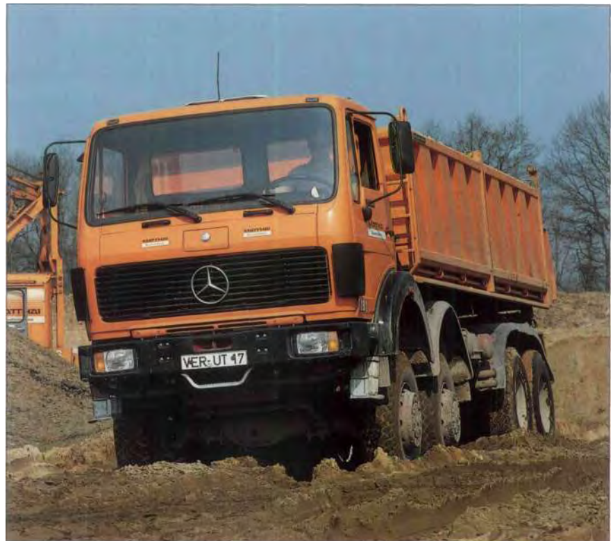
The four-axle truck line comprises chassis with capacities of 32 to 48 tonnes gross vehicle weight, with engine performances from 206 to 261 KW (280-334 HP) and wheel bases from 4.10 to 6.50 meters.
