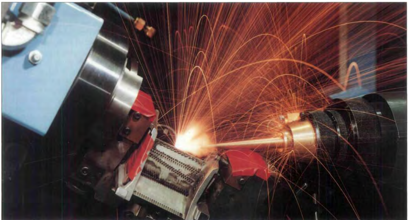
Laser beam drilling of cooling air apertures in a heat-resistant turbine blade.
