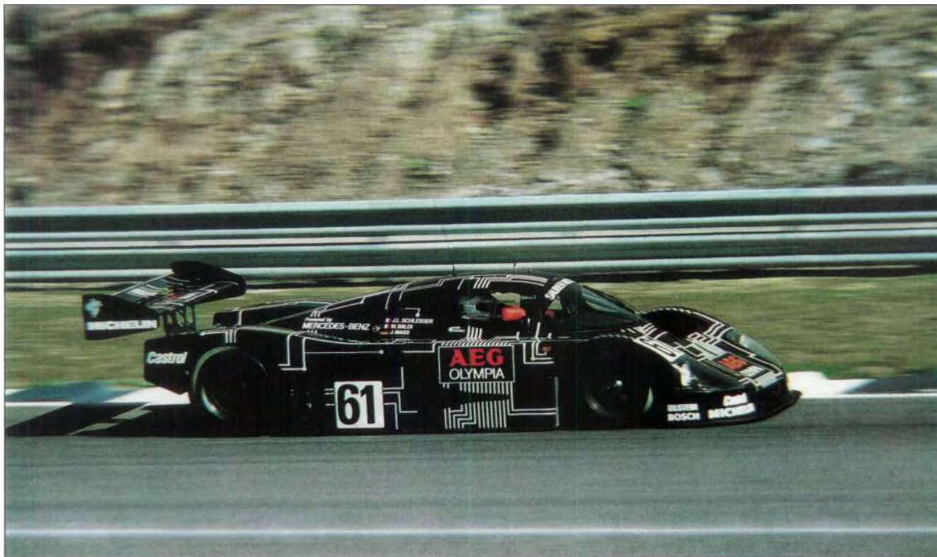
The SAUBER Mercedes C9 finished the first race of the 1988 season in Jerez, Spain, as the winner. The Group C racing car has an 800-horsepower, five-liter Mercedes V8 engine.
