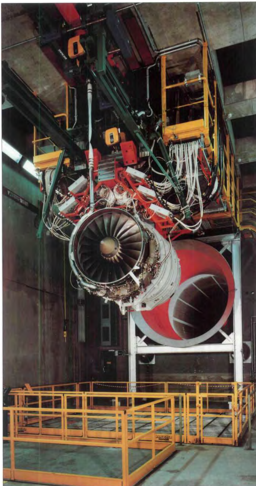
This test stand for large jet engines with a thrust of up to 300 k is equipped with the most modern measuring systems.
