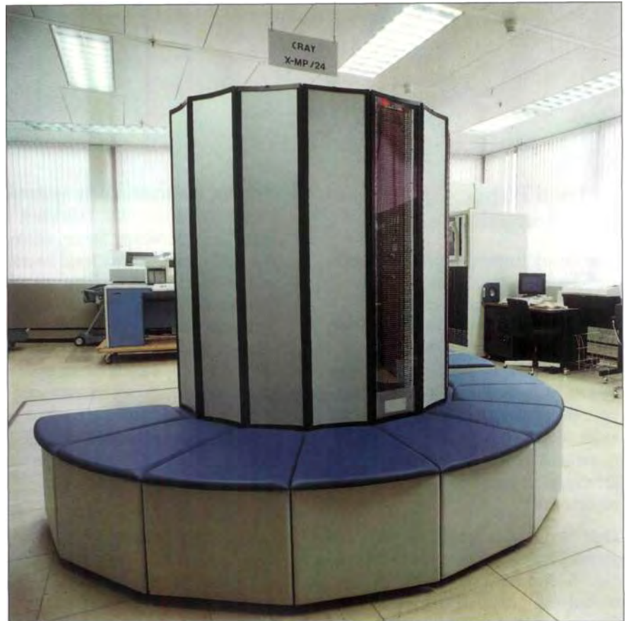
CRAY XMP/24: super computer with a capacity higher than that of 20,000 personal computers.
