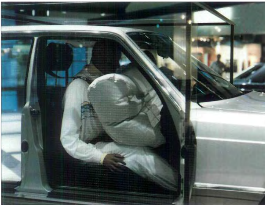
Since the end of 1980, a supplemental restraint system for the driver has been offered: the airbag in the steering wheel. More than 400,000 Mercedes automobiles have been thus equipped. Now, with an airbag for the front passenger too, in combination with the standard seatbelt tensioners, Daimler-Benz offers a comprehensive system to reduce the risk of injury in head-on collisions.
