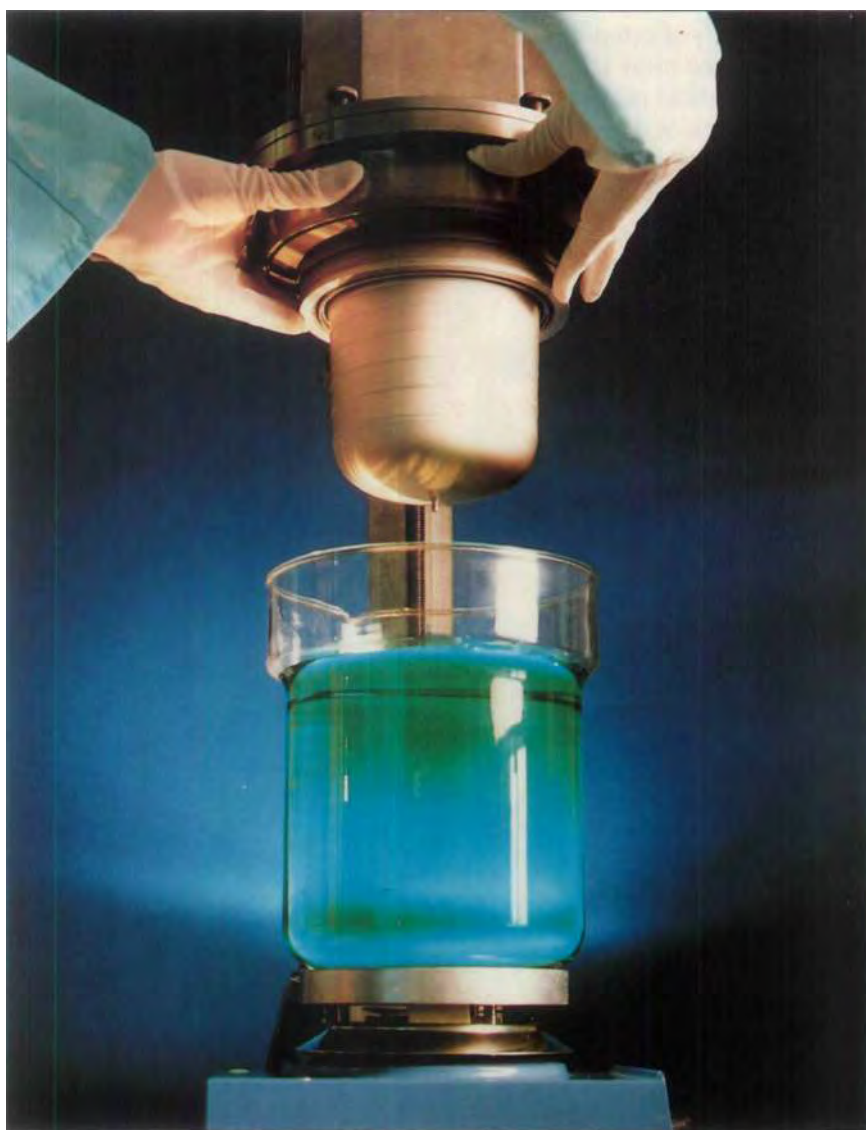
Nickel-plating a collector for a high-performance traveling-wave tube from AEG for use in a satellite. Traveling-wave tubes are the key components for the high transmitting power - up to 260 watts - of these satellites.
