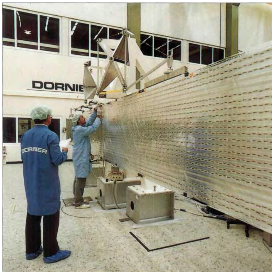
The SAR (Synthetic Aperture Radar) antenna of the European Earth Reconnaissance Satellite, ERS-1, is made of carbon-fiber reinforced plastic.
