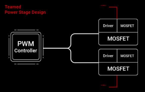
The teamed architecture allows two power stages to work in tandem to provide more power to the CPU.
