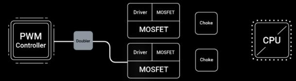
Each VRM component serves a specific purpose. PWM controllers and phase-doublers control the circuit, and the power stages do the heavy lifting from an electrical and thermal standpoint. That's why ROG Maximus XII Formula utilizes 16 power stages. The power stage sits at the top of Infineon's lineup and features a low RDSON to reduce switching and conduction losses, helping to improve overall thermal headroom.
