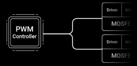
While doublers help extend the number of effective phases, they do so at the cost of a processing delay.
