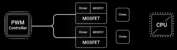
The MOSFETs within the power stages generate the most heat as they are responsible for voltage conversion and delivery to the CPU from the 12V EPS connector.
