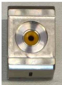
Fig. 57: Piston seal installed in the displacement chamber
