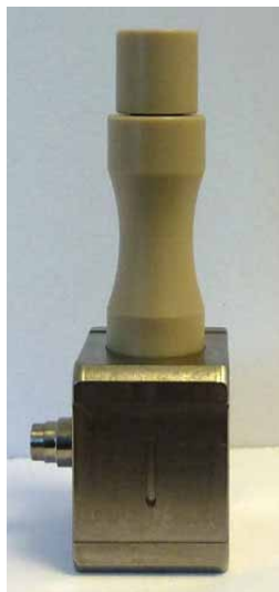
Fig. 56: Installing the replacement seal using the seal handling tool
