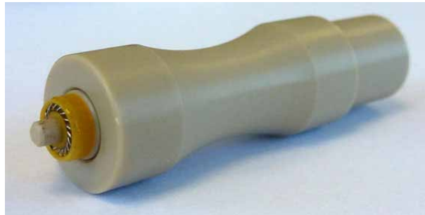
Fig. 55: Piston seal positioned on the seal handling tool (open seal side facing away)
