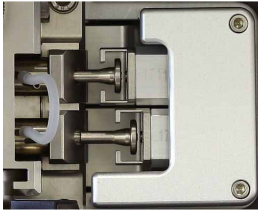
Fig. 44: Pistons without piston retaining springs
