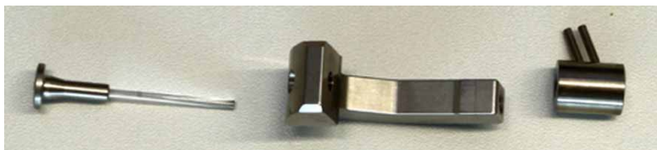
Fig. 59: Holding hook disassembled
