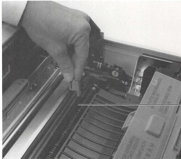
Figure 6-14 Cleaning the discharging pins
