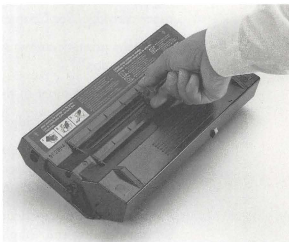
Figure 7-6 Cleaning the primary corona wire
