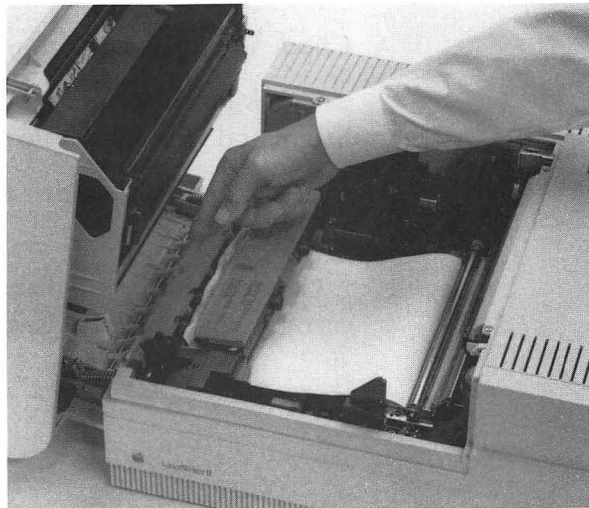
Figure 7-4 Removing jammed paper from the fixing rollers
