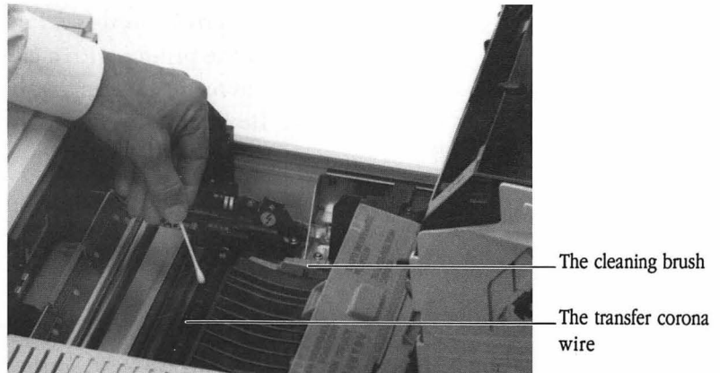
Figure 6-15 Wiping the transfer corona wire
