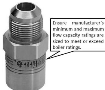
Figure 48 - Excess Flow Valve (EFV)
