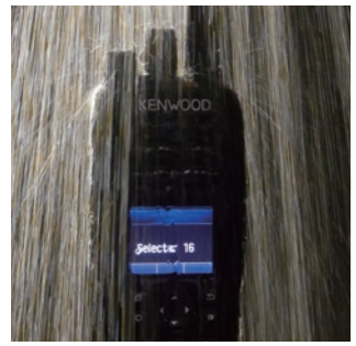
Heavy Rain Test
