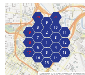
12.5 kHz digital system At a total of 2150 sq. miles coverage: 5.8-mile radius per site / 21 site total
