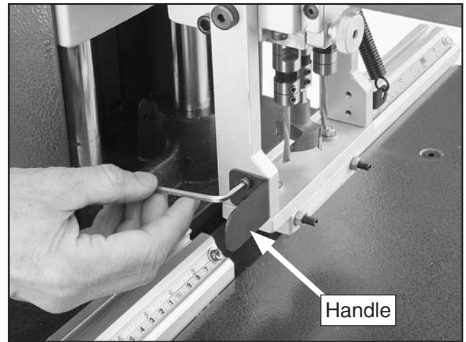
Figure 19. Installing swing arm handle.
