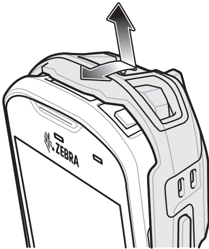
Figure 133 Lift Boot Over Device
