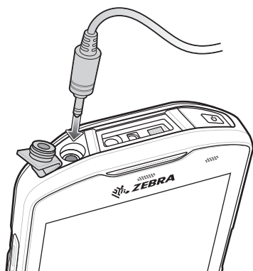
Figure 147 Audio Adapter Installation
