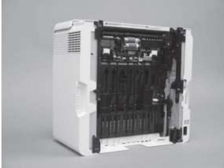
Figure 6-18 Place the printer bottom-side face forward
