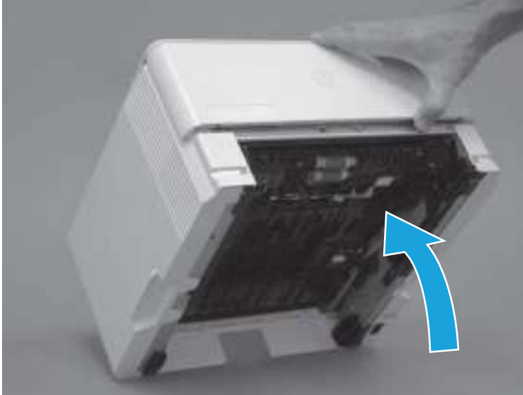
Figure 6-17 Tilt the printer backward
