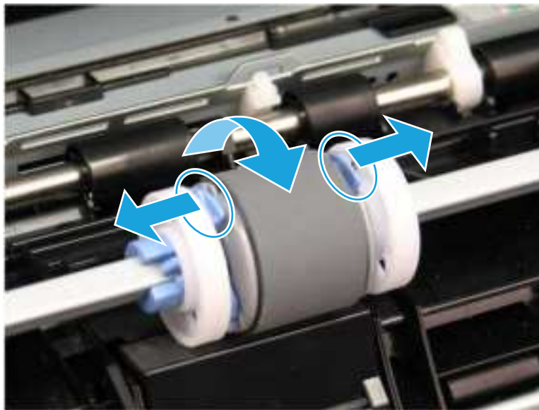
Figure 6-12 Release the roller
