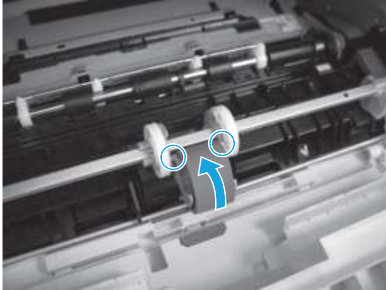
Figure 6-15 Install the roller
