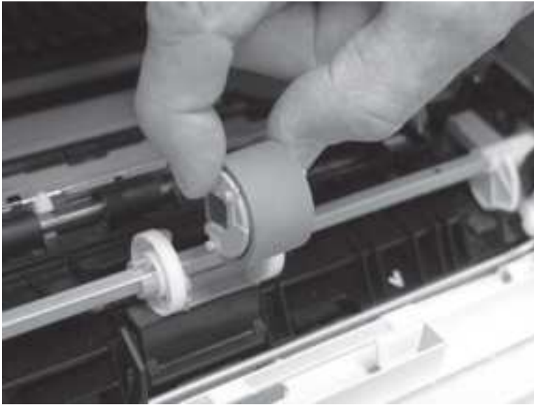
Figure 6-13 Remove the roller
