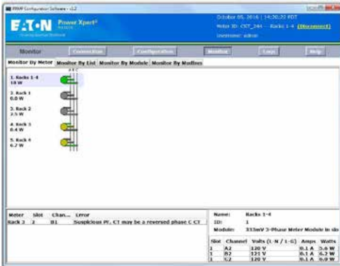
Figure 30. Software in Monitor Mode to View the Metering Data for Each Tenant Meter.
