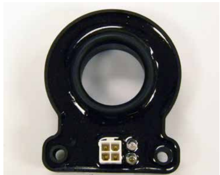
Figure 42. 2x2 Load Facing Side of a 100 mA PXMP-CS250 Solid Core Current Sensor Showing 4-Pin Connector Compatible with External PXMP-SCXX Sensor Cable Locator, and Clamp Active Alarm LEDs.
