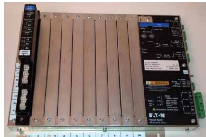
Figure 37. Module Installed in the Meter Base Assembly.
