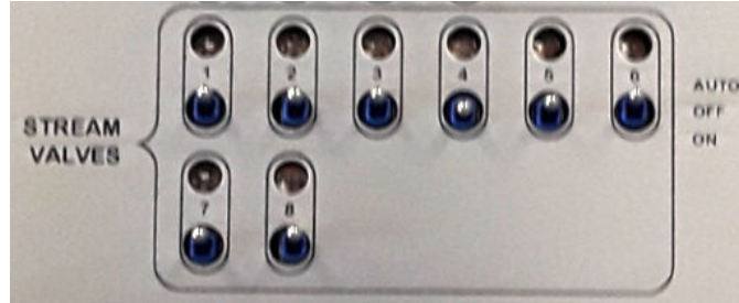
Figure 2-4: Stream Valves Switches
