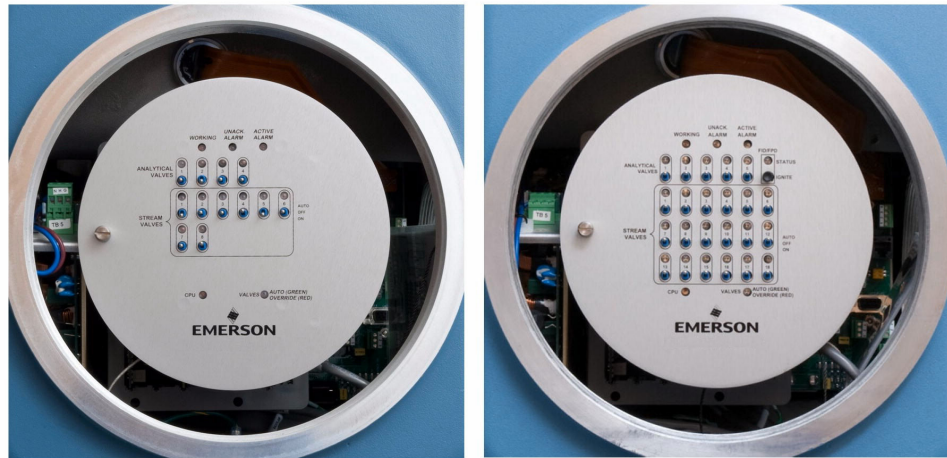
Figure 2-2: 8-stream switch panel (left) and 18-stream switch panel (right)
