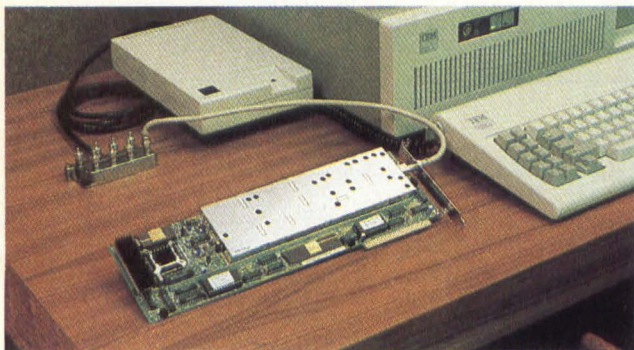
The IBM PC AT and PC Network hardware: Sytek supplies the adapter card and IBM is a licensee of Sytek's LocalNet/PC protocols.
