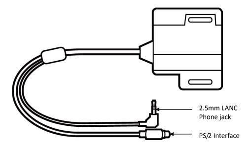
This unit allows you to operate the JVC camera with the MCU-100J unit at a distance of up to 300m away from the camera.
